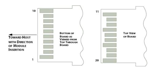
**Figure 3: Module Contact Assignment**
