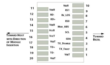
Figure 2: Module Interface to Host
