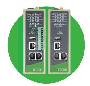
The new IIoT edge computing gateway provides uninterrupted Internet access for machines over ubiquitous 3G/4G wireless networks and multiple broadband services. With powerful edge computing capabilities, comprehensive security protection and wireless services, InGateway902 can support device networking of up to 10,000 levels, providing high-speed data channels in the true sense of device informatization.
