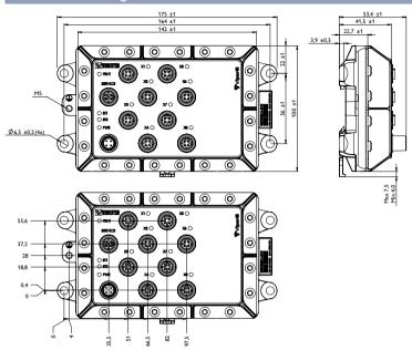
Weight 0.9 kg Degree of protection IP65
