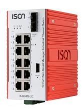
The IS-DG410 Series are full Gigabit web-smart managed 10-port Ethernet switch with 2GTX/FX port that provide easy to access, plug-n-play Gigabit ports for applications; The cost-effective IS-DG410 Series web-smart managed switches can be easily used in factory production line or embedded into machine system. The IS-DG410P Series switches also support some useful function by default for network traffic optimization, such as QoS and storm protection.
