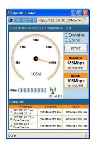
SpeedFlex<sup>™</sup> is a unique wireless performance test tool integrated within the ZoneFlex<sup>™</sup> family of centralized controllers that measures the Wi-Fi throughput of associated wireless LAN clients.
