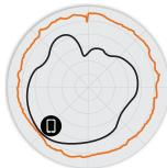
Figure 4. T811 2.4GHz Elevation Antenna Patterns
