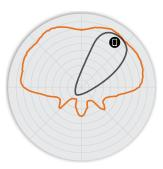
Note: The outer trace represents the composite RF footprint of all possible BeamFlex+ antenna patterns, while the inner trace represents one BeamFlex+ antenna pattern within the composite outer trace.
