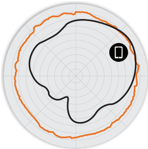
Figure 2. T710o 2.4GHz Azimuth Antenna Patterns
