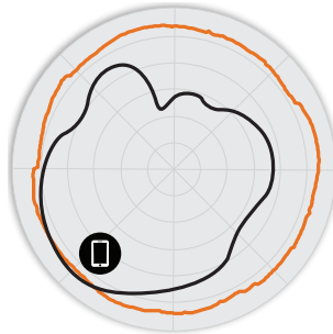
Figure 3. T710o 5GHz Azimuth Antenna Patterns
