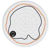
Figure 3. T310d 5GHz Azimuth
