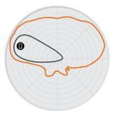
Note: The outer trace represents the composite RF footprint of all possible BeamFlex+ antenna patterns, while the inner trace represents one BeamFlex+ antenna pattern within the composite outer trace.
