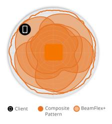
Figure 2. R720 2.4GHz Azimuth Antenna Patterns
