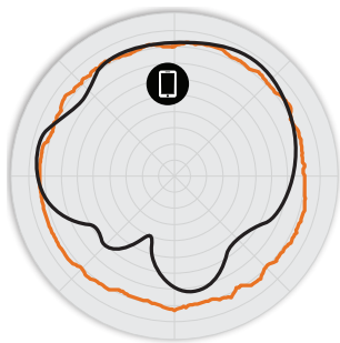
Figure 2. R500 2.4GHz Azimuth Antenna Patterns
