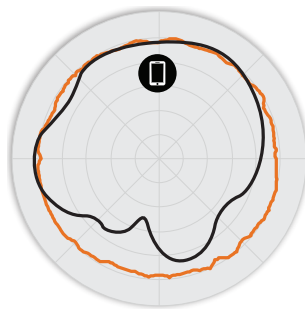
Figure 3. R500 5GHz Azimuth Antenna Patterns
